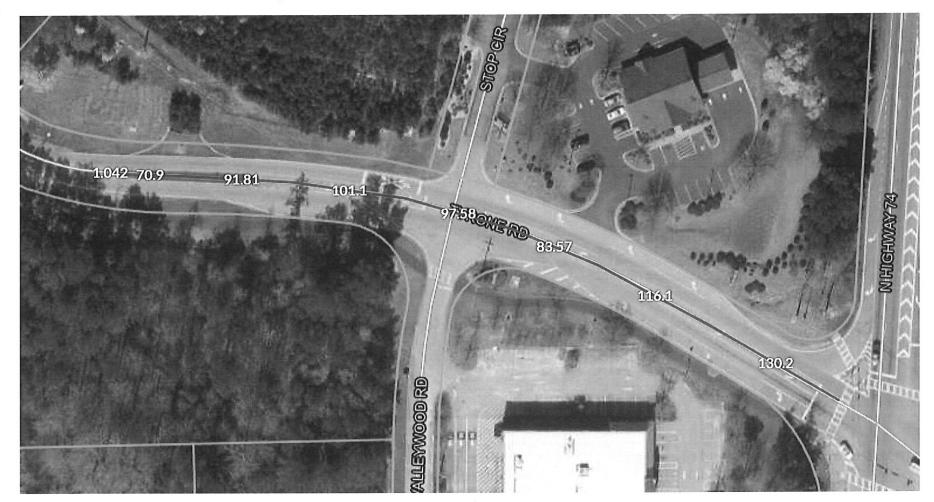
**Roadway Description:** Two lane roadway, including turning lanes, accel lanes, and decel lanes. (approx. 0.13 CLM). **Detail:** Roadway connector between SR-74 ROW and western end of planted median.
