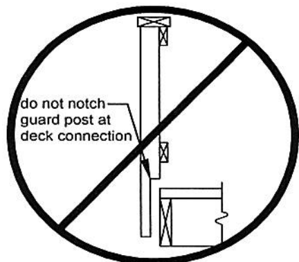
FIGURE 28: NOTCHING AT GUARD POSTS
